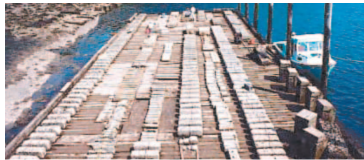
Concrete test samples, some of them several decades old are subjected to the elements as part of various research programs at the US Army Corps Engineers National Weathering Exposure Station for Concrete and Concrete Materials at Treat Island, Maine.
